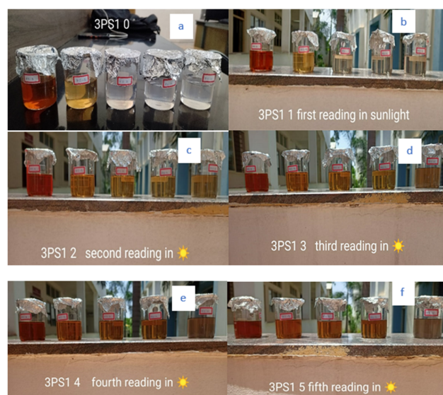
Figure 5: Formation of silver nanoparticles by varying concentration of the of tea extract at different interval of time in presence of sun light, (a) initial (b) 1 min (c) 2 min (d) 3 min (e) 4 min (f) 5 min.
